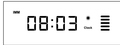
Clock mode, where 'clock' indicator is lit
